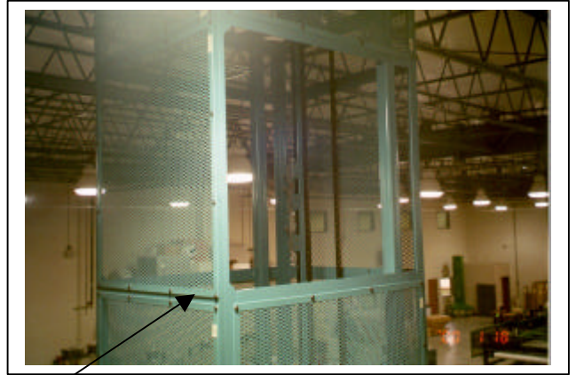
Flat Metal Edging Protects Expanded Metal
